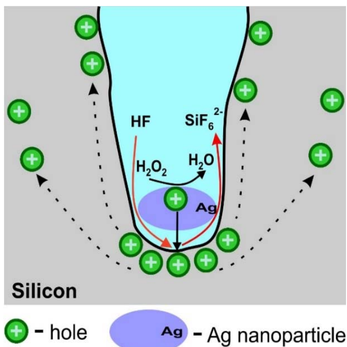
Figure 2.1. Sketch of the MACE process, where \text{H}_2\text{O}_2 is reduced to \text{H}_2\text{O} at the noble metal particles and the holes are injected into Si that leads to the dissolution of Si as \text{SiF}_6^{2-} species.
