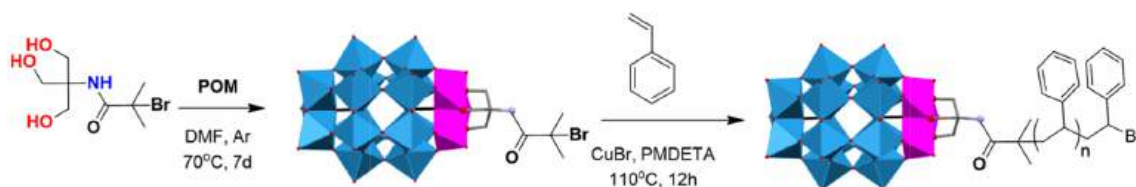
Fig. 31. The first example of POM-polymer hybrid synthesis based on a trivanadium-substituted WD POM.
