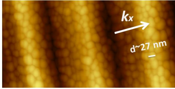
Figure 3.1. AFM topography image of \sim 7 nm thick non-percolated Au layer deposited on a corrugated template of P \sim 290\text{nm} exhibiting the randomly oriented Au grains with diameter d \sim 27 nm. ( k_x direction is along the spatial corrugation vector) 218 .
