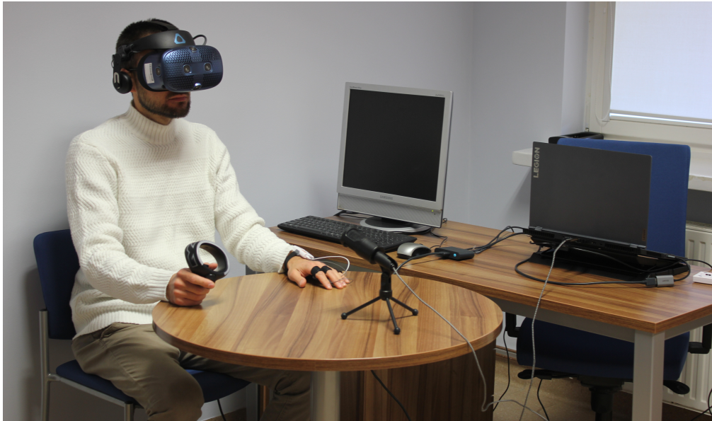
Figure 1: Experimental setup for participants. Participants wore VR headset and were placed in a virtual café environment. Psychophysiological data were recorded using the Shimmer3 GSR device, visible on the participant’s left hand, while the VR controller was held in the right hand. A microphone was positioned in front of the participant to enhance the illusion of real-time voice interaction.
