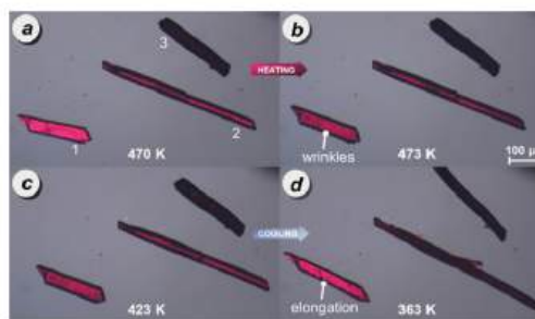
Fig. 2 Hot stage microscopy of PDI-C 6 crystals during the heating cycle: (a) phase I at 470 K, (b) transition from phase I to phase II at 473 K; and during cooling cycle: (c) phase II at 423 K, (d) transition from phase II to phase I at 363 K, reshaping the crystals. Additional images are provided in Fig. S18 and S19 of the ESI†.
