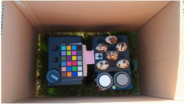
FIGURE 1 Set for photographing eggs: custom-made supporter on a tripod with pits for eggs, grey standards and scale bar. All set was surrounded on the sides by a box to prevent Japanese quail Coturnix japonica blown eggs from shaking due to wind.
