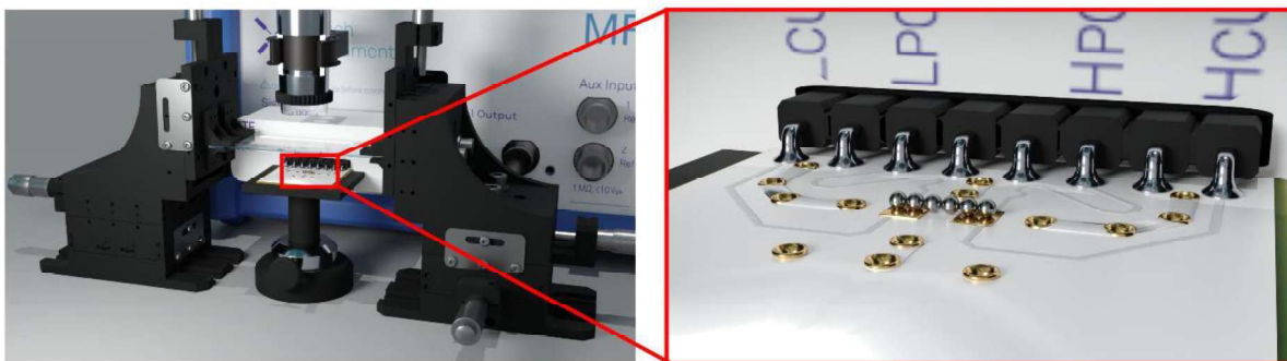
Figure 8. Experimental setup for electrical characterization of compressed particle chains. The impedance was measured using a precision impedance analyzer (Zurich Instruments, MFA, 5 MHz) connected to the manufacturer's impedance test fixture (MFITF). A custom-designed two-terminal PCB carrier with low capacitance and minimal parasitic losses was used to hold the sample. The carrier consisted of two copper pads ( 1.5 \times 1.5 mm, \sim 30 \mu m thick) separated by a \sim 1.4 mm gap, across which the particle chain was deposited (right). Compression was applied in situ using a 5 mm thick glass slab mounted on a translation stage (left), which allowed for precise displacement control and simultaneous optical monitoring of chain deformation by the camera positioned above the compression slab.
