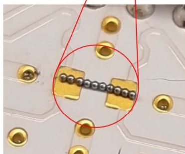
Figure S4. We used impedance spectrometer from Zurich Instruments (MFIA) to measure the real part of impedance. The particle chain was deposited on a 2T DUT (device-under-test) carrier with two copper pads (thickness of \sim 10 \mu\text{m} , and the gap between the pads \sim 16 \text{mm} ) plugged into an MFITF Impedance Test Fixture, which ensured very accurate measurements of impedance, especially at low values close to the limit of the instrument ( \sim 0.1 \text{m}\Omega ). The experimental setup enabled in-situ monitoring of electrical impedance during particle chain compression.
