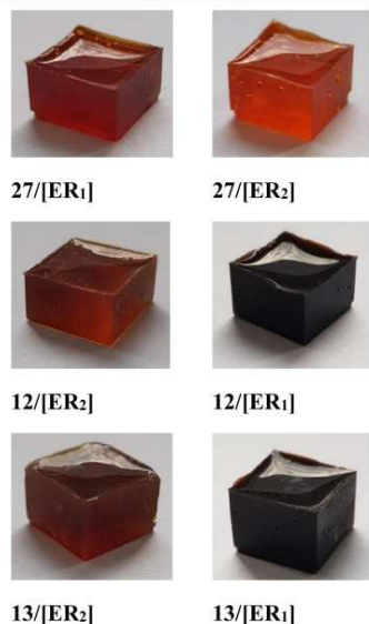
Figure 6. Shore samples of cured epoxy resins with dicyanamide DABCO ILs (curing systems as described in Table 4).
