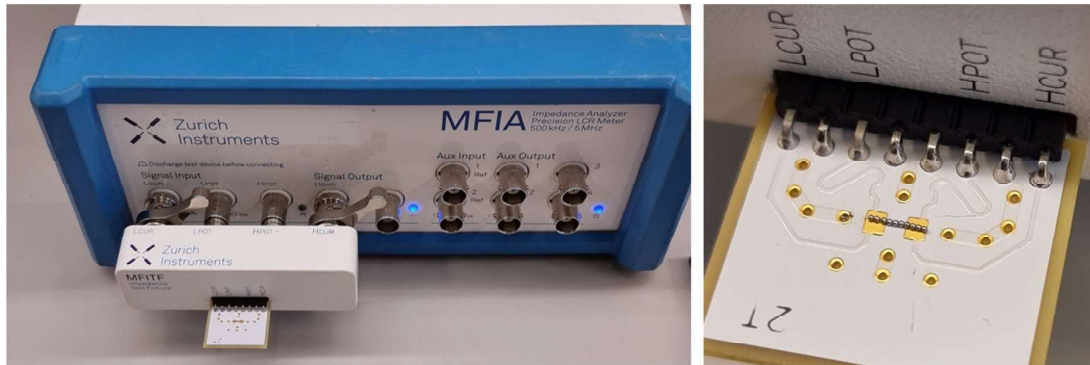
Figure S2. An MFIA impedance spectrometer from Zurich Instruments was used to measure the particle chain resistance. The particle chain was placed on a 2T DUT (device-under-test) carrier with two copper pads, approximately 10 \mu\text{m} thick, and a gap of around 16 mm between them. The carrier was connected to an MFITF Impedance Test Fixture, ensuring high precision in impedance measurements, particularly for low values near the instrument’s sensitivity limit ( \sim 0.1 \text{ m}\Omega ). This experimental setup allowed real-time monitoring of electrical impedance during the compression process of the particle chain. The PCB carrier was selected to minimize parasitic effects and damping by eliminating the need for lead wires, facilitating the study of the electronic properties of particle chains. The equipment was calibrated using an open-circuit test (measurement of a device with infinite impedance) and a short-circuit test (measurement of a device with zero impedance). This setup achieves the measurement accuracy comparable to the four-wire method, as the influence of lead wires is practically eliminated, and the contact resistance is significantly smaller than the resistance of the particle chain (see also Figure S5 ).
